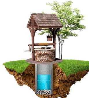
A cross-section diagram of a traditional well. It shows a vertical shaft (Ствол) leading down to a water-bearing layer (Верховодка). A blue cylindrical pipe at the bottom is labeled 'Гравий' (gravel). The top part of the shaft is labeled 'Оголовок' (head). A wooden structure with a roof, labeled 'Глиняный замок' (clay cap), sits atop the well head. The surrounding area is shown with green grass and brown soil.
